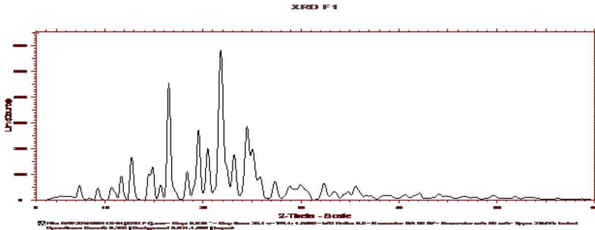
Figure 16: XRD of Liquid SEDDS
