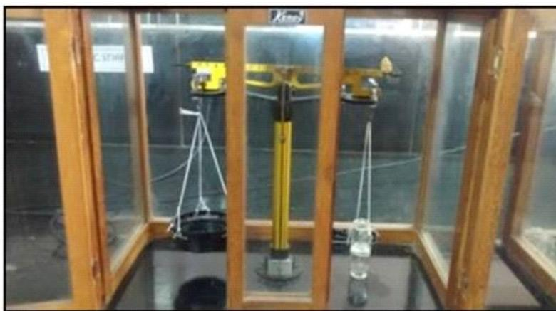
Figure 1: Modified balance for Mucoadhesion study
